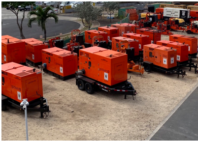
Dri-Prime Pumps for Sewer Bypassing & Dewatering
